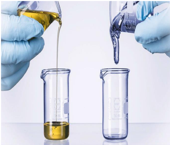
Fig. Different fluid flow behavior in a same type of glass tube
