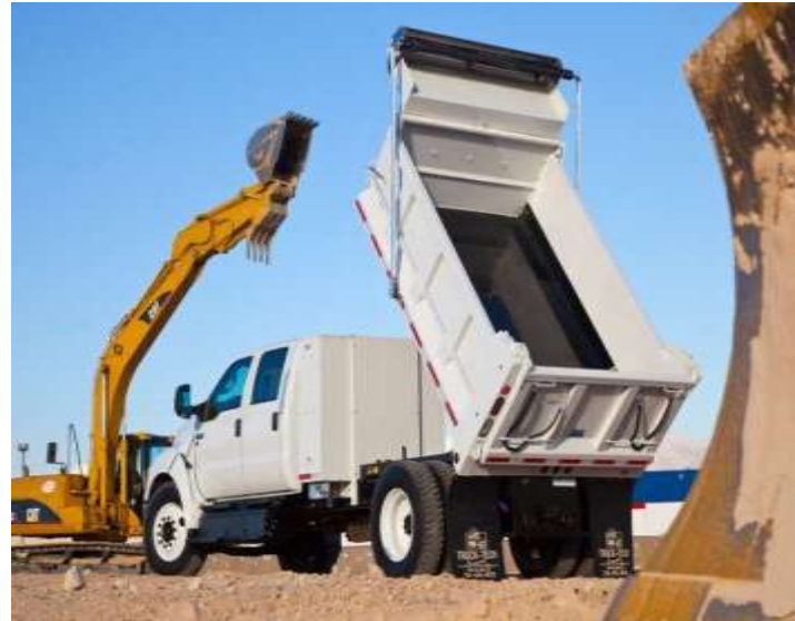
Rear dump truck
