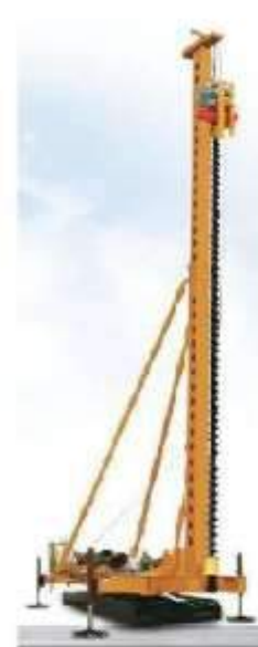
CFG pile driving machine
