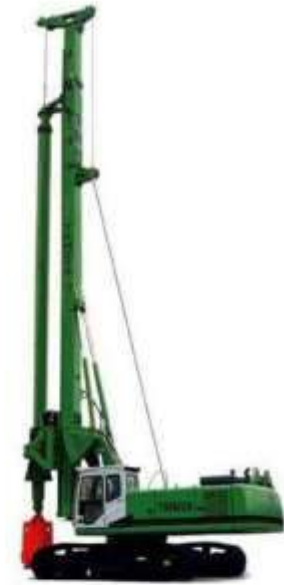
Rotary drill rig
